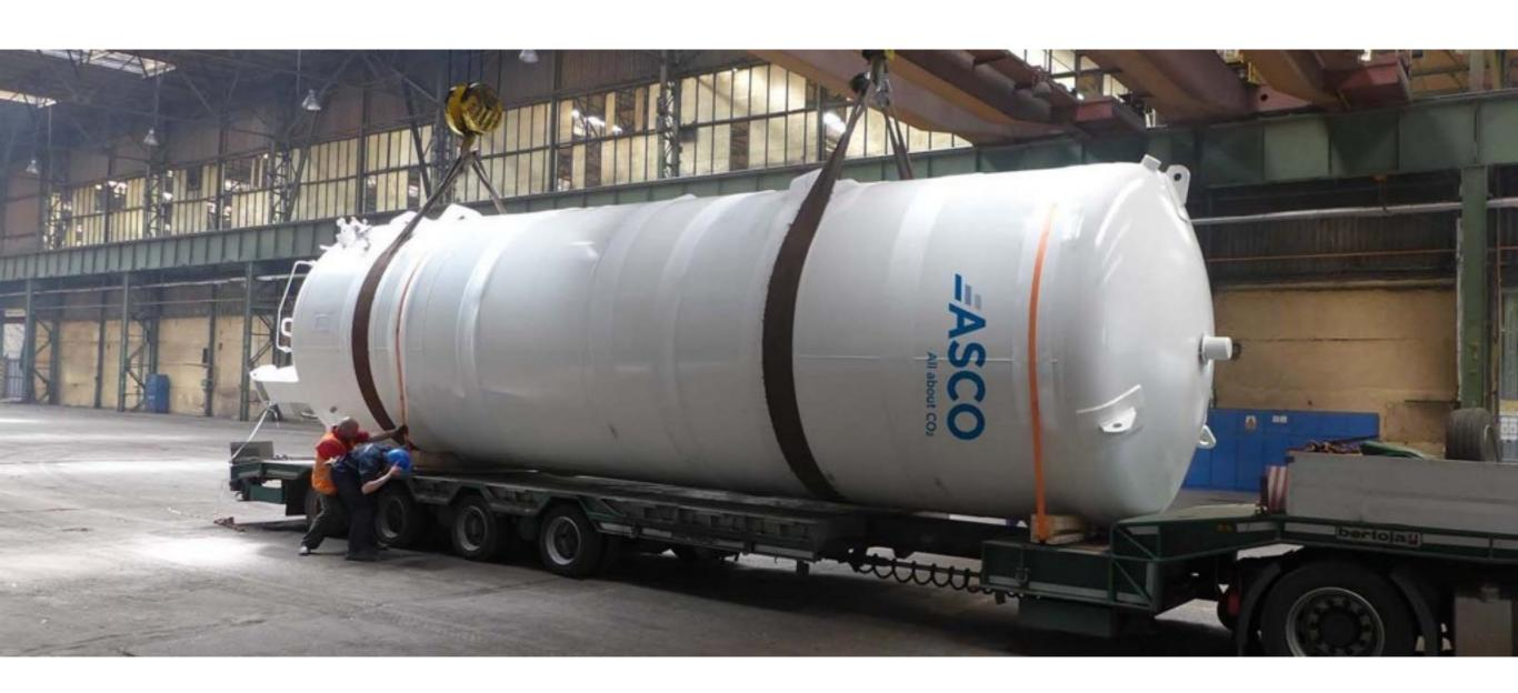
Typical 30 ton Tank for storage liquid CO2
